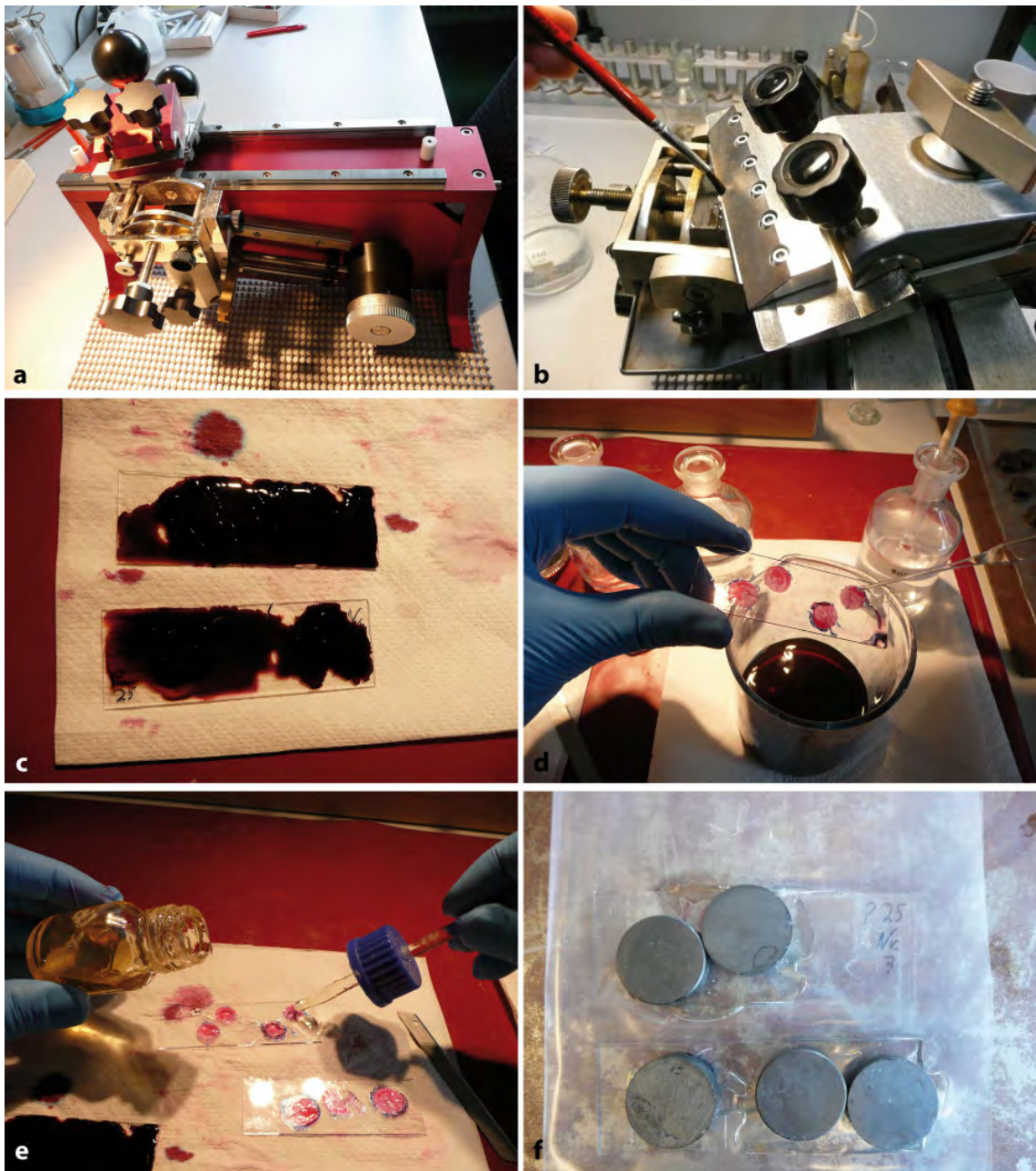
Fig. 2.4 Different working steps of sectioning and staining: (a) Core microtome without sample (b) Facilitating thin cutting by wetting the sample with a brush (c) Sections covered with Safranin/Astrablue-mixture (d) Leaching out of the colour with a pipette of water/ethanol (e) Dropping of Canada balsam onto the slides (f) Slides under magnets on an iron plate, ready for the oven.
