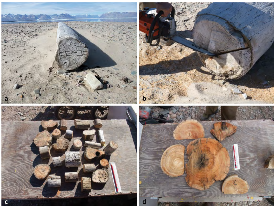
Fig. 2.2 Pictures of the sampling in Greenland, Scoresbysund: (a) Logged stem with a mark, probably from a logging company at the beach in Scoresbysund (b) Sampling of a driftwood-stem with the chainsaw (c) Collection of raw small samples (d) Collection of raw large samples (Pictures taken by Willy Tegel).
