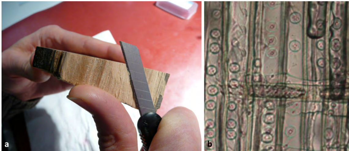
Fig. 2.5 Cutting by hand: (a) Radial cutting with the box cutter (b) Resulting section ( Larix sp. ) on an object slide with some drops of water under the microscope (Reflected light microscope with a magnification of 400).
