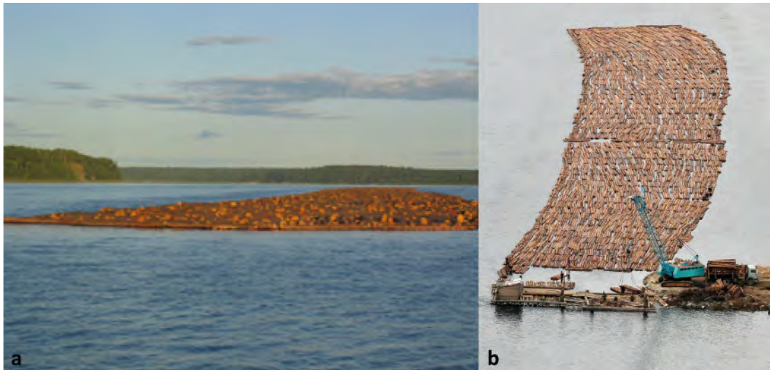
Fig. 4.7 Timber floating on the Angara river: Stems are tied together into rafts for the transport down the river (a) Source: http://www.ldkl.ru/images/bigimage12.jpg (b) Source: http://msnbcmedia.msn.com/j/MSNBC/Components/Photo/_new/pb-110728-timber-rafts-eg.photoblog900.jpg .
